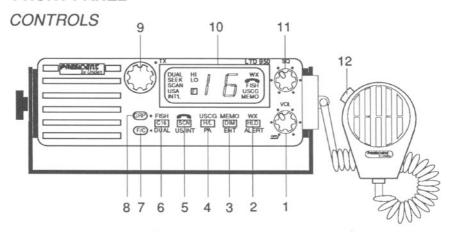
VOL (On/Off/Volume) - Turns the LTD 950 On or Off and varies the audio output.
